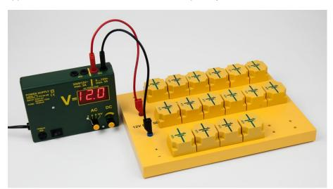
Each individual slot in the charging plate is protected against overvoltage by an internal series resistor.
