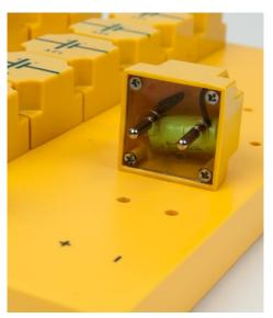
The charging plate is now supplied with 12 V DC. Here, too, the correct polarity must be observed.
